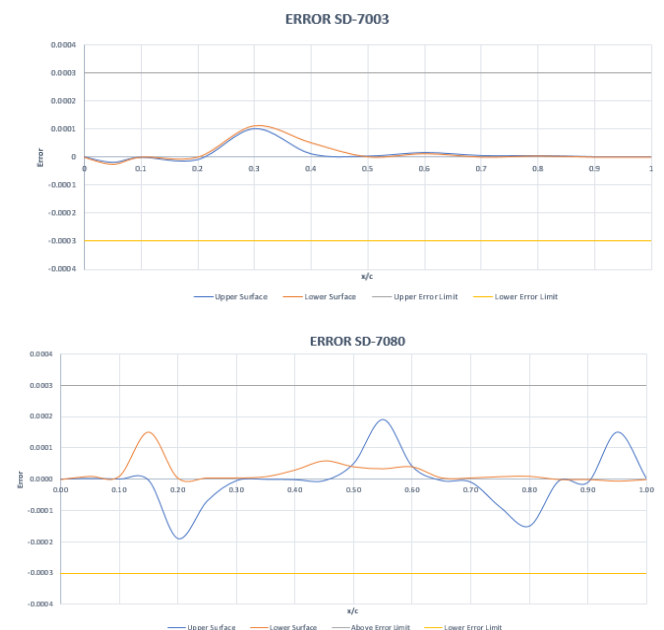
Fig. 9. Error comparison of parametric and original airfoils
