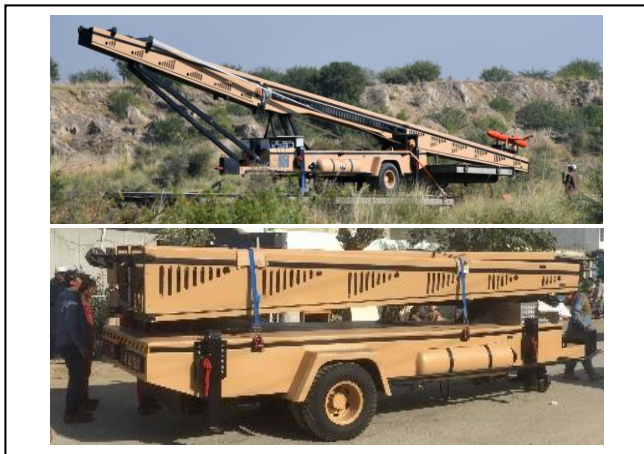
Fig. 1. Pneumatic catapult launcher in fully extended configuration (top) for aircraft launch, and stowed configuration (bottom) for transportation.
