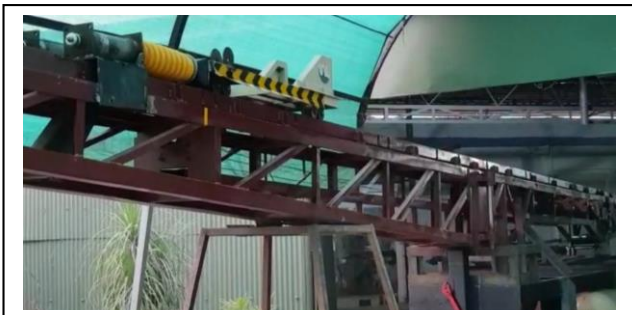
Fig. 8. Spring mounting and impact pad assembly attached on front rail segment
