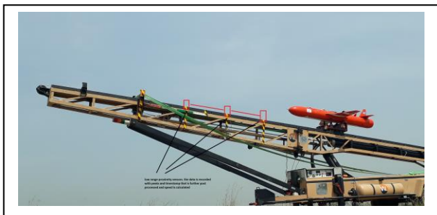
Fig. 12. Proximity sensors installed at marked locations.
