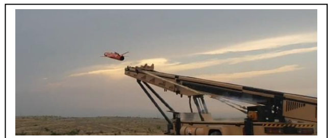
Fig. 10. At the moment of launch, the shuttle is arrested into the belt seen as flexible elements below the rail.
