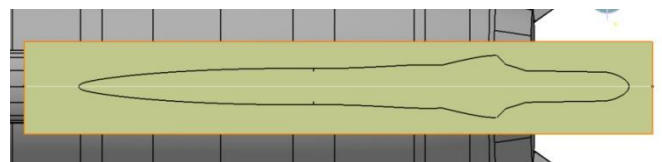
Figure V-g: Dorsal fin airfoil extracted from CATIA model
