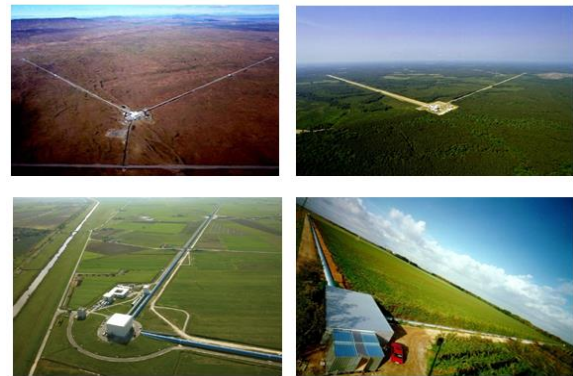
Fig 2: Aerial photographs of the LIGO observatories at Hanford and Livingston, VIRGO at Italy and GEO at Germany. The lasers and optics are contained in the white and blue buildings. From the large corner building, evacuated beam tubes extend at right angles for 4Km in each direction (the full length of only one of the arms is seen in each photo); Credit: LIGO laboratory [14].
